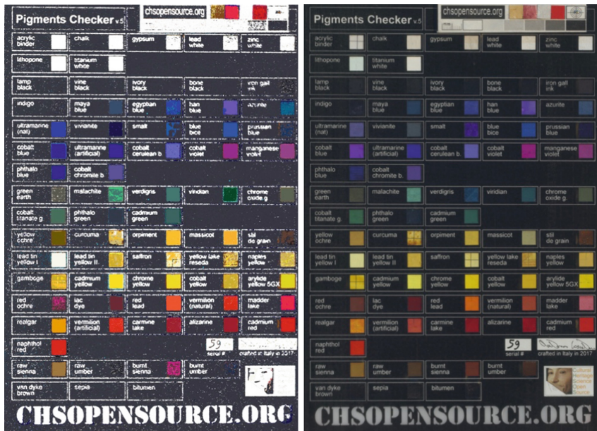
Fig. 5. CHSOS Pigment Checker (2018). RGB generated image (left) and pigment classification XPECTRALTEK platform (right). © SRAL
