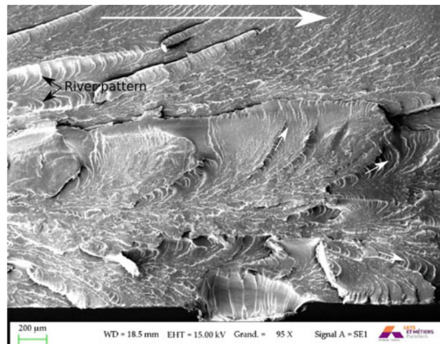
Fig. 8.6 Observation by electron microscopy of the propagation zone of the fracture surface of sample B5. The large white arrow at the top indicates the main direction of propagation of the macro-crack front. The three small white arrows indicate the propagation directions of several micro-cracks. Characteristic river patterns in multiphase polymers with high heterogeneity can be observed
