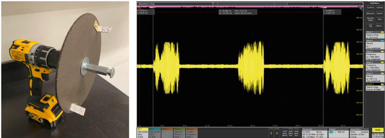
Fig. 14.5 Trial velocity measuring system used (left) and a screenshot from oscilloscope measurements of the setup (right)
