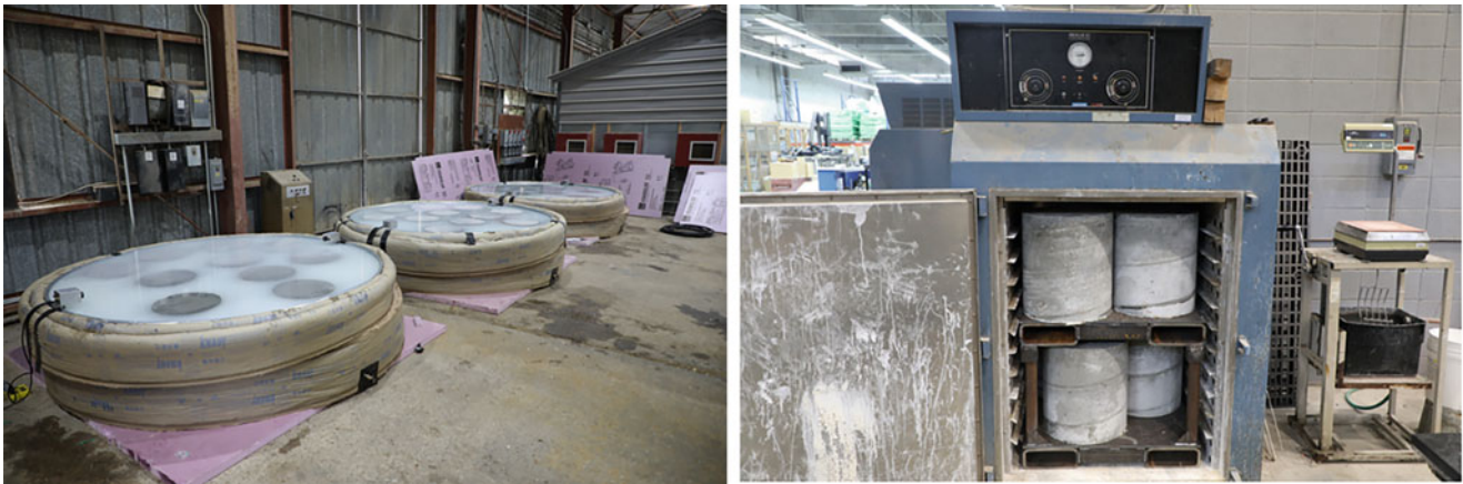
Fig. 11.2 Concrete curing protocols for saturated specimens (left) and oven-dried specimens (right)
