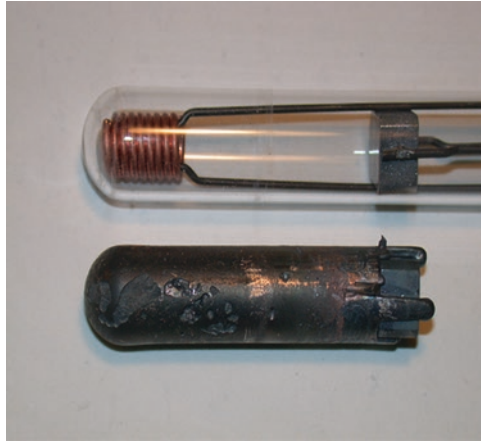
Fig. 4. Internal probe construction before and after a sampling sequence; “single-grab” design [2].
