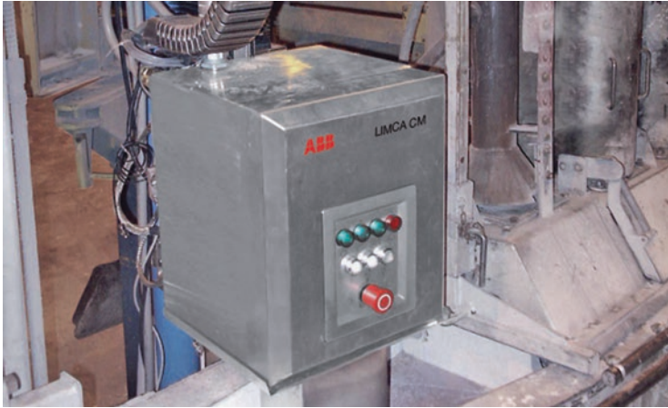
Fig. 2. Liquid metal cleanliness analyzer for continuous monitoring of melt quality (LiMCA CM ©) [6].
