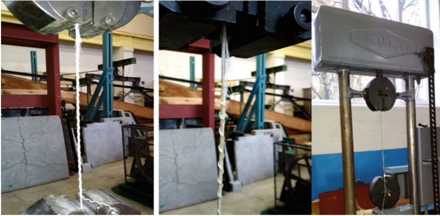
Fig. 13 General view of tests of samples from fiberglass reinforcement
