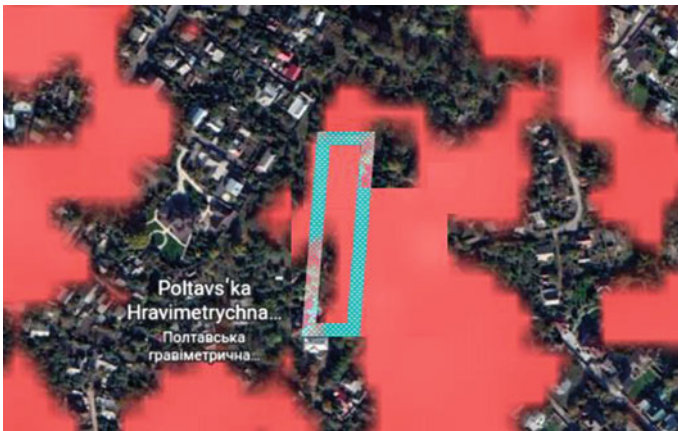
Fig. 6 Geodetic polygon (□) of the Poltava Gravimetric Observatory (city of Poltava, Ukraine) on the Google Earth map with the display of vertical displacements between the two images from 08.10.2020 to 06.04.2021
