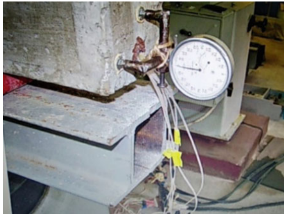
Fig. 6 General view of fixing the indicator and lead wires of the resistance strain gauges in the test specimen–concrete beams
