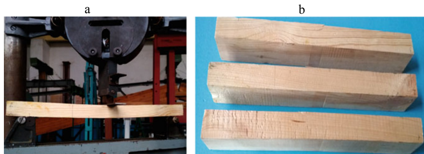
Fig. 2 a–overall view of the wood bending test; b–test specimens after destruction
