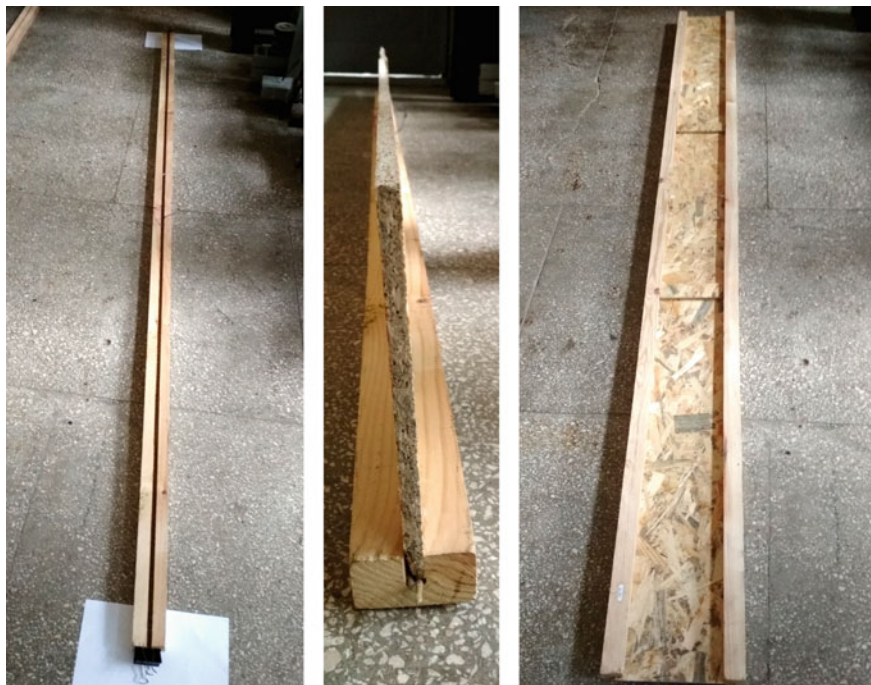
Fig. 24 Preparation for gluing and a glued sample of the fourth series
