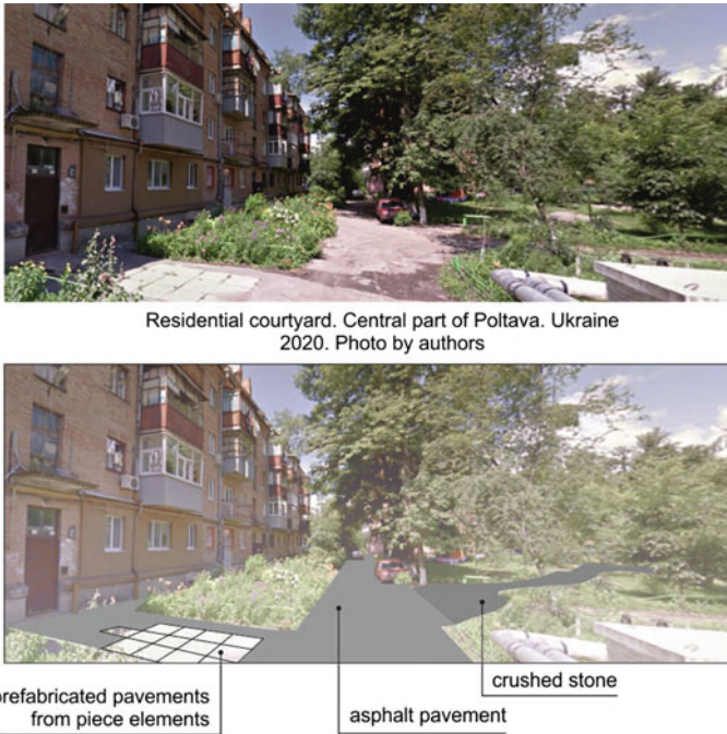
Fig. 6 Analysis of the elements of the payment of one of the yards of residential buildings of 1950–1980 Poltava (Ukraine). Source photoby authors
