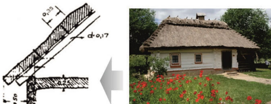
Fig. 2 Traditional Ukrainian technology of covering roofs with reeds. Source Scheme—by authors, photo—[18]
