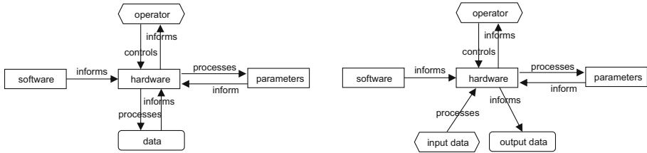
Fig. 2. A model of an IT system with indicated parameters. Data may be considered as a unified input and output component (left), or separate input and output data components (right).
