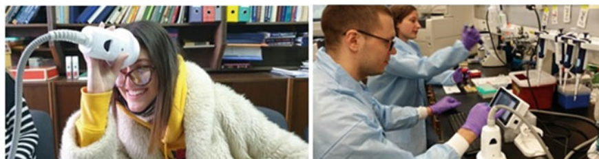
Fig. 16 OMIS as “mirror mimicry” device based on reflection may characterise tissues in vivo (left) and in vitro (right). It can be used in lab, clinic, home, working place, etc. Three main processes are: taking images (PROCESSING), data analysis (ANALYSING) and result presenting (DIAGRAMS or REPORT), presenting on right side of picture
