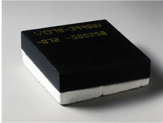
Fig. 6 Silica Space Shuttle thermal protection (TPS) tile, ca. 1980. Science Museum London [49]
