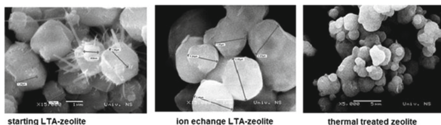
Fig. 4 SEM micrographs of zeolite LTA topology (starting, ion exchange and thermal treated)
