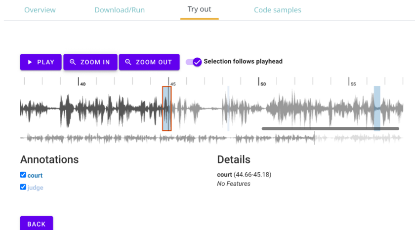
Fig. 2 Example of the word “court” having been detected as a keyword using HENSOLDT ASR
