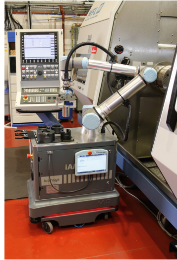
Fig. 1. Collaborative robot in action inside the AMRC gear center
