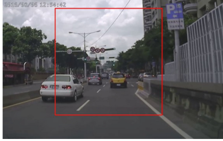
Fig. 7. The input images with resolution of 1280 \times 800 are cropped with a 612 \times 612 ROI for further processing.
