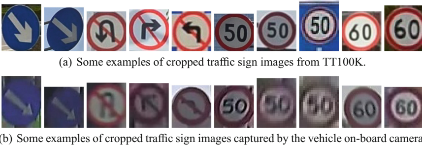
Fig. 5. Examples of cropped traffic sign region from TT100K and vehicle on-board camera. The images captured by the on-board digital video recorder are generally blurry and noisy compared to most TT100K dataset images [2].
