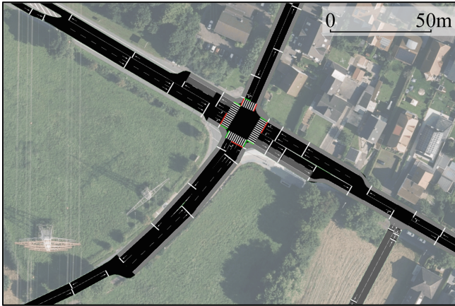
Fig. 12. SUMO-GUI embedded in a bird's-eye view of a real world TLS controlled intersection in Schloß Neuhaus [27].
