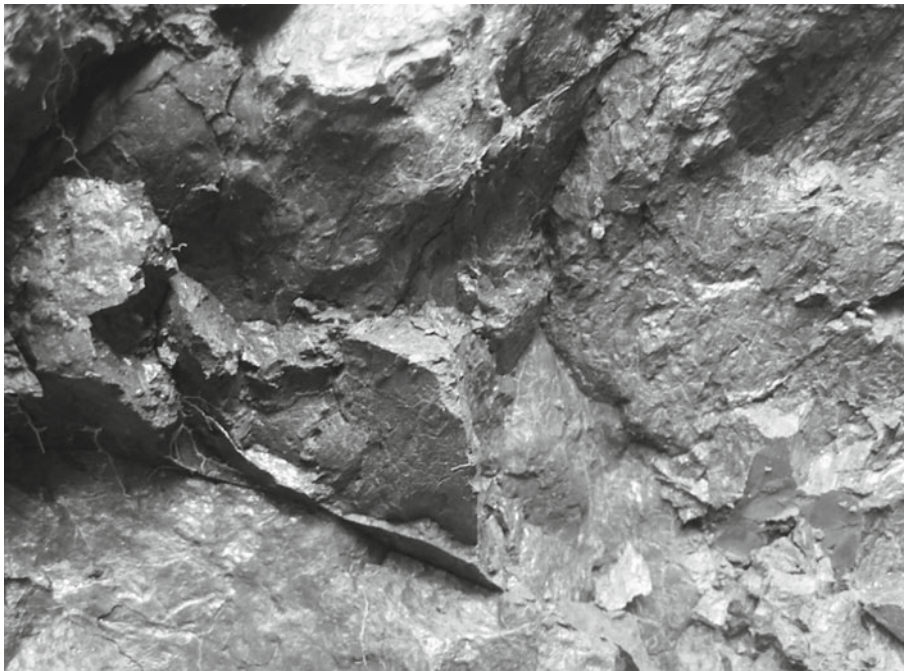
Fig. 7.5 Slickenside formation of Vertisols Ener and Enamore, southern Ethiopia (Photo courtesy of Alemayehu Regassa)
