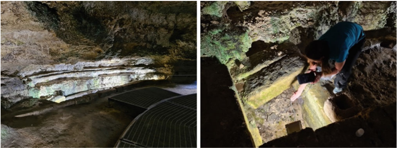
Fig. 7 Details of the springs at Fonte Pliniano : left, water dripping from the wall at the contact between calcarenites and the silty and clay interlayers; right, checking the water parameters with a field probe
