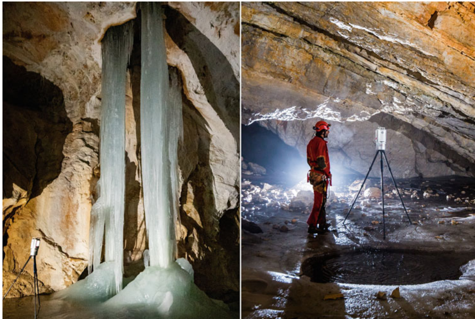
Fig. 2 Laser scanning in an ice chamber in Snežna jama na planini Arto (left) and Velika ledena jama v Paradani (right)
