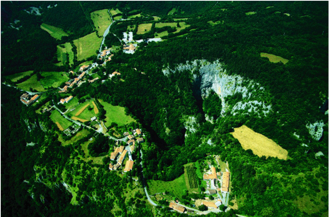
Fig. 4 Due to the denudation of the karst surface, the ceiling of an empty cave passage thinned and collapsed, creating consecutive collapse dolines; the Škocjan Caves (Slovenia), UNESCO heritage site. Photo Škocjan Caves Park
