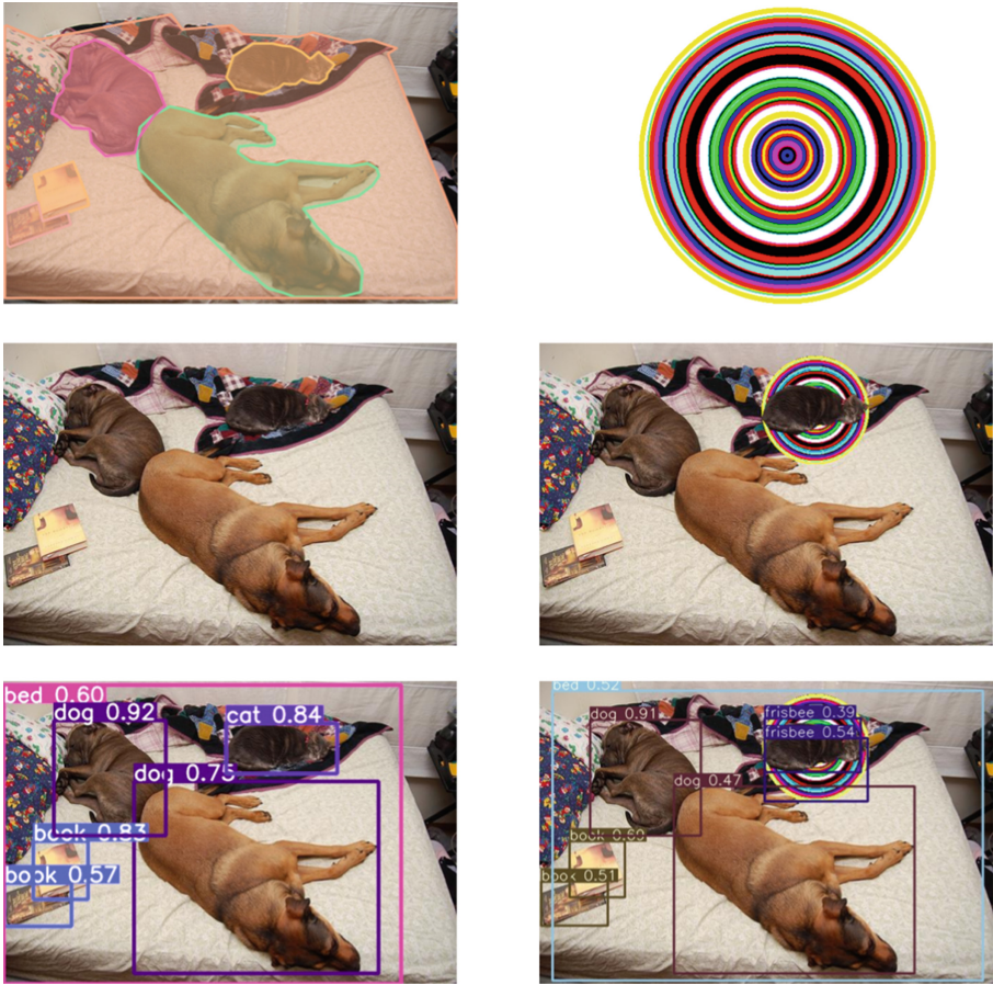
Fig. 1. The universal background image and attack schematics. Top: the left column is the result of instance segmentation, and the right column is the universal background image generated on YOLO v3 model. Middle: the left column is the clean image, and the right column is the adversarial example obtained by placing the universal background image under the target object cat. Bottom: the left column is the detection result of the clean image, where the target object cat is normally detected with high confidence of 0.84, and the right column is the detection result of the adversarial example, where the target object cat is misclassified as a frisbee.
