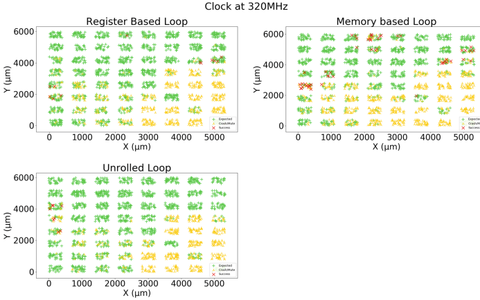
Fig. 5. EMFI results of all three tests at 320 MHz (PLL enabled).
