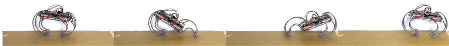
Fig. 11. Selected screenshots of the video recordings. Here Morphology M_B is executing motion sequence S_B , which was the fastest morphology-motion-pair from the second test series.
