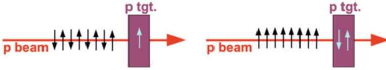
Fig. 12.2 Left: Polarized proton target with proton beam unpolarized by averaging over spin states. Right: Polarized proton beam with proton target unpolarized by averaging over spin states
