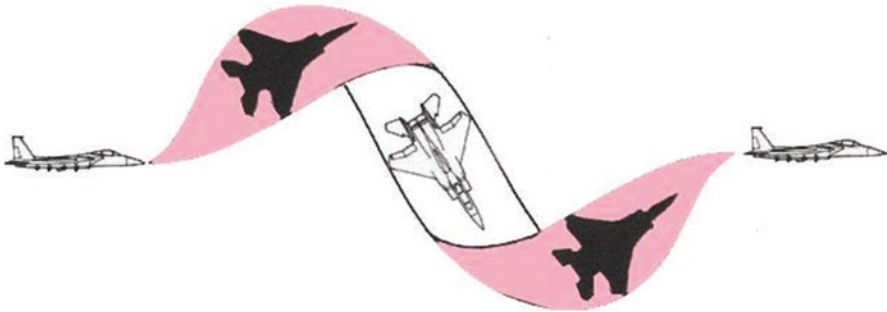
Fig. 3.5 A “Barrel Roll” is a rotation around the x -axis combined with some up pitch and down pitch around the y -axis in a corkscrew path
