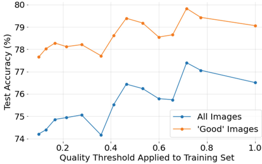
Fig. 4. Classification accuracy of the downstream model trained on different datasets filtered as per varying pre-defined continuous quality thresholds on two different test sets: unfiltered (blue) and 'good' (categorical quality) images (orange). (Color figure online)
