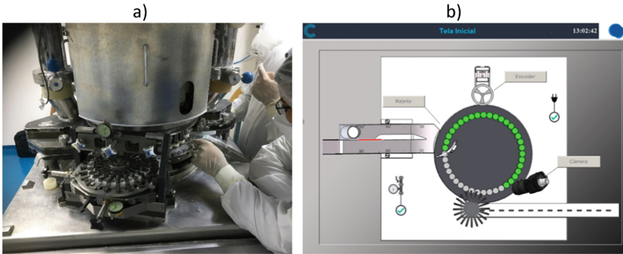
Fig. 1. a) Real world powder compressor; b) powder compressor Lean digital twin. Finished prototype. (Source: the authors)
