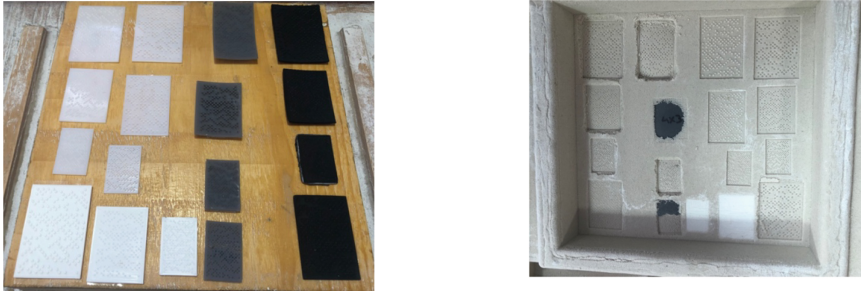
Fig. 5. Mold pattern with tags inserted (left); the drag (lower half of the mold) after drawing the pattern (right).
