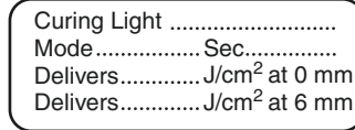
Fig. 5.9 Label for monitoring energy delivered by a LCU during regular maintenance, at the College of Dentistry, University of Iowa. (Courtesy: Dr. Steve Armstrong, University of Iowa)
