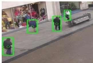
Fig. 5. Detection of people with bounding box
