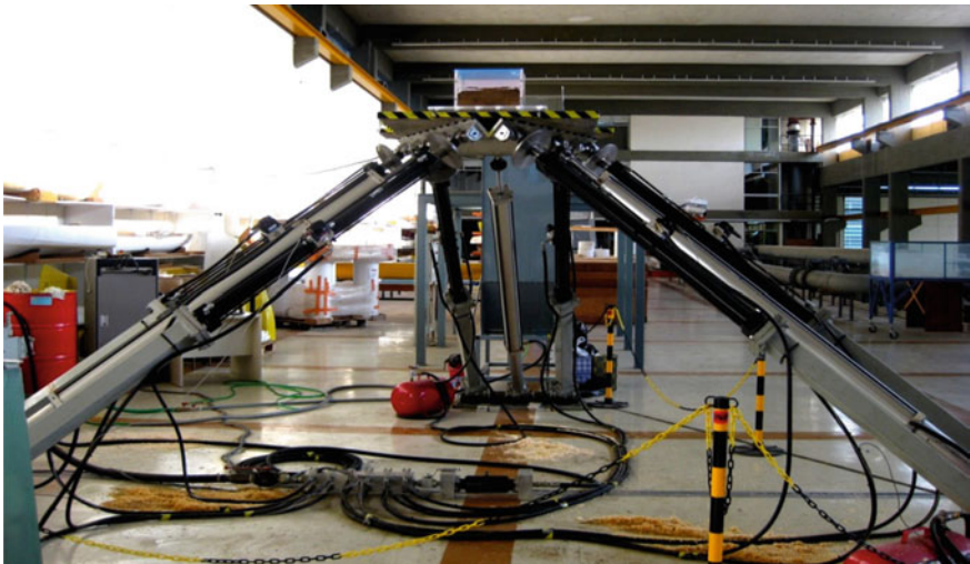
Fig. 1 The shaking table equipment of NTUA's School of Naval Architecture and Marine Engineering
