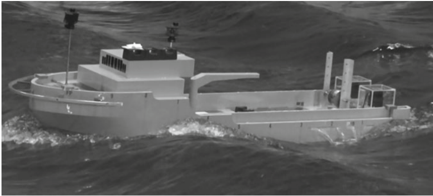
Fig. 2 Free-running model experiment of the OSV in stern quartering waves executed in 2015
