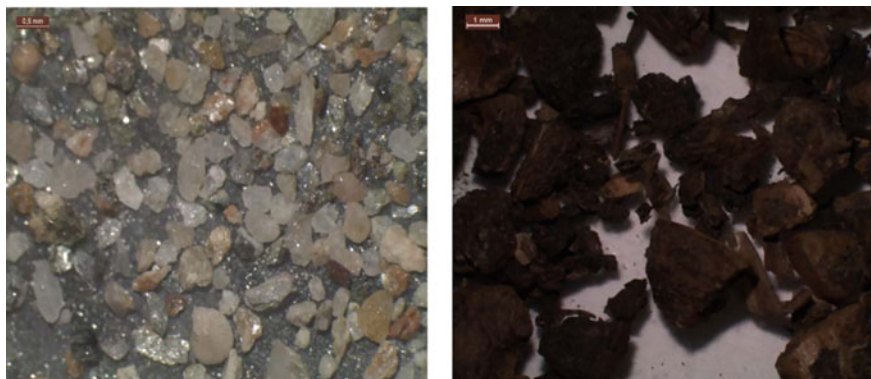
Fig. 2 Visualisation of the samples of sand (left) and olive pomace (right) through optical microscope
