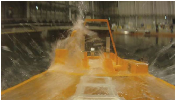
Fig. 9 Shipping water on upper deck
