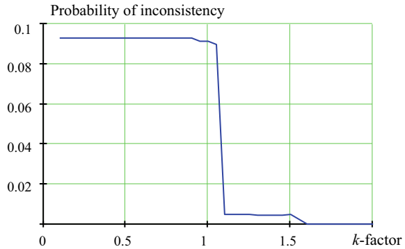
Fig. 8 The probability of inconsistency for the alternative level 2 criterion as a function of the degree of applicability of the linear roll assumption ( k -factor) for a standard of 0.06
