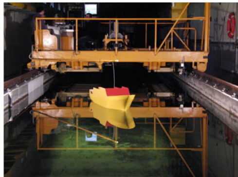
Fig. 2 Hull bodyplan (left) and scale model towing tank tests arrangement (right)
