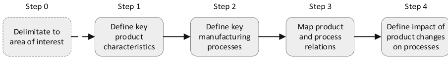
Fig. 1. The five steps and sequence of the proposed method for changeability assessment.
