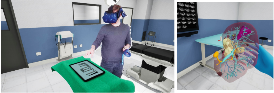
Fig. 3. Our virtual operating room with a point cloud avatar of a remote user on the left and an interactive virtual liver on the right.
