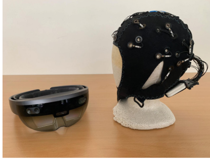
Fig. 5. Illustration of the apparatus used in the developed prototype. (Left) A Microsoft HoloLens AR headset and (Right) an mbt Smarting EEG headset.
