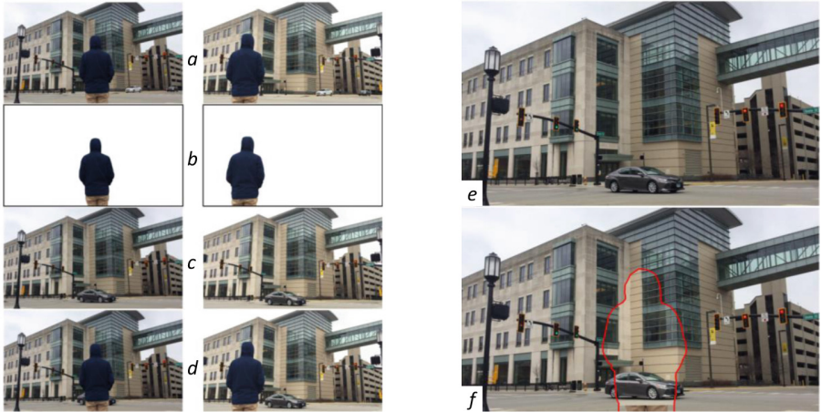
Fig. 11. Comparison of our disocclusion method to a ground truth transparency effect: (a) primary and secondary frames with occluder, (b) extracted occluder, (c) primary and secondary frames without occluder, (d) extracted occluder b inserted into frames c, (e) ground truth transparency effect, (f) output of our algorithm.
