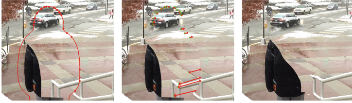
Fig. 7. Local mapping need (left), implementation (middle), and result (right). Left: disoccluding using only the global mapping results in discontinuities where near objects cross the occluder contour, e.g. where the sidewalk and handrail cross the red line in the left image. Middle: the local mapping connects primary frame salient contour points (red points) to their correspondence in the secondary frame (green points); the local alignment offset is larger for near objects. Right: disocclusion with continuity at occluder contour.
