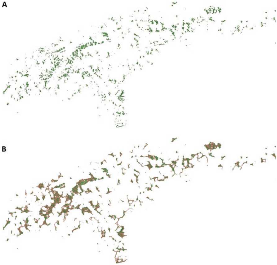
Fig. 3 Saint-Malo's lagoon LiDAR maps of the (a) midslope ridges' class and (b) the graph-based network of that class thresholded at a 200 m distance
