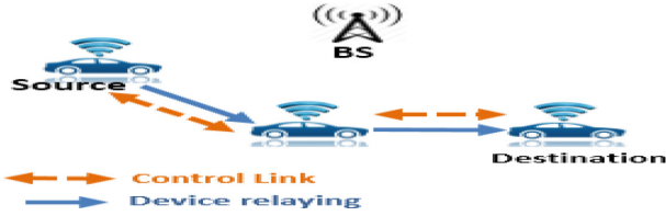
Fig. 2. D2D communication with self-controlled links.
