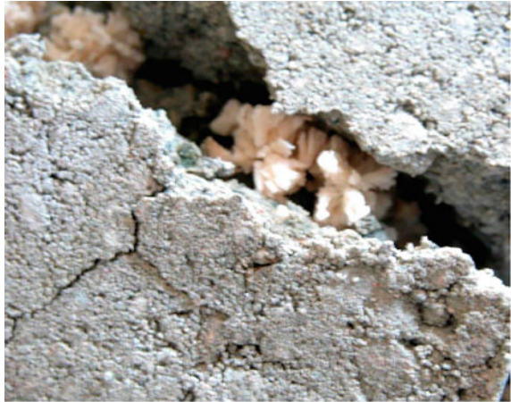
Fig. 11 Formation of secondary ettringite [67] reproduced with permission from ISCOWA
