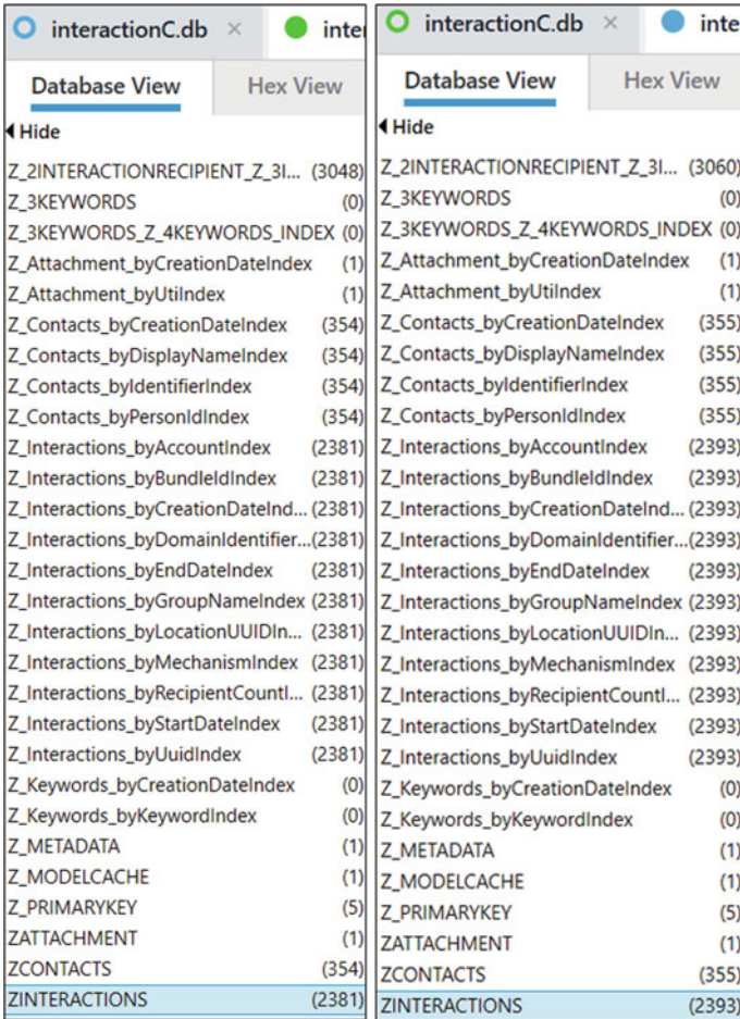
Fig. 6.26 iPhone X comparison of ZINTERACTIONS table in the interactionC.db database
