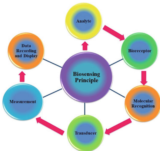
Fig. 6.1 Basic principle of nanobiosensors
