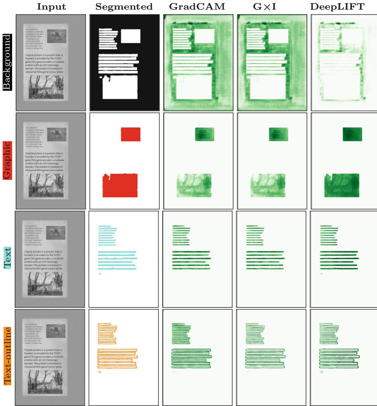
Fig. 3. Image segmentation and explanation outputs. From top to bottom, each row corresponds to the attribution of the four classes: background, graphic, text and text-outline, respectively using the three XAI methods: GradCAM, G \times I and DeepLIFT.
