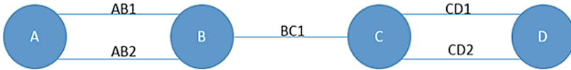
Fig.1. Multigraph with four nodes: A, B, C, D and five connections (edges).
