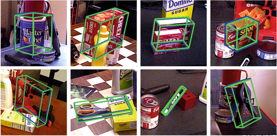
Fig. 3. Qualitative results on YCB-Video dataset. Example images demonstrate how our algorithm handles occlusions, objects in various poses, and lighting conditions. Depicted are the following objects: 002_master_chef_can, 003_cracker_box, 008_pudding_box, 010_potted_meat_can, 035_power_drill, 040_large_marker, and 051_large_clamp. The blue bounding boxes show the ground truth poses, whereas the green ones correspond to the estimated poses. For better visualization the regions of interest were cropped. (Color figure online)
