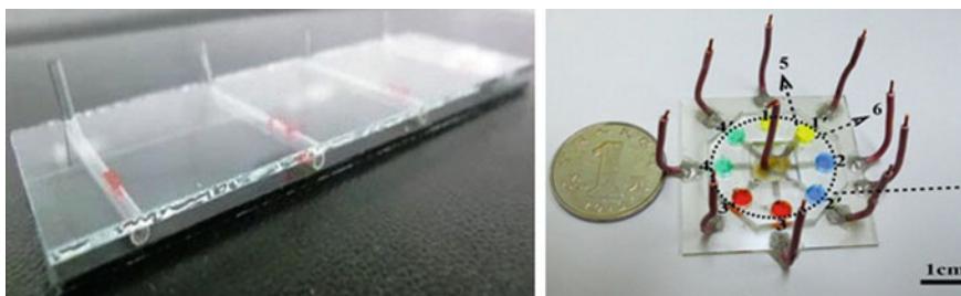
Fig. 3 Images of the microdevices that take advantage of loop-mediated isothermal amplification (LAMP) reaction for TB diagnosis through genotyping: left, picture of the glass capillaries for turbidimetric evaluation of the precipitate formed after LAMP reaction in the capillaries; right, indium tin oxide electrodes used for redox detection based on methylene blue reaction with M. tb DNA. It contains eight isolated electrochemical microchambers, and an inlet hole and an outlet hole are drilled on each microchamber. (Adapted with permission from [34] and [35])
