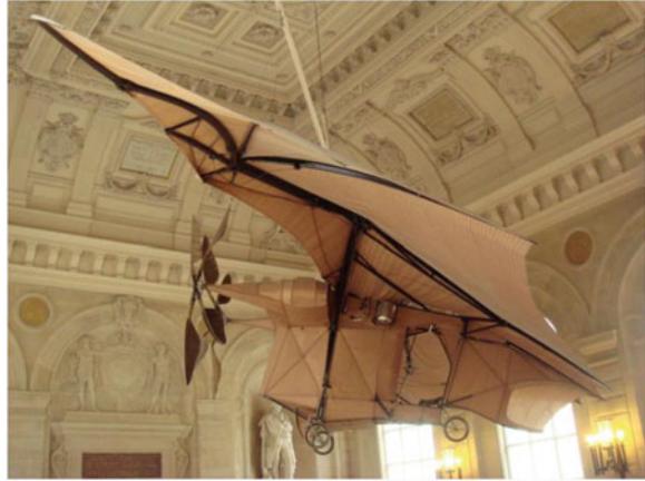
Fig. 7.12 The bird-like aircraft Avion III designed by Clément Ader, a French aviation pioneer in the late nineteenth century
