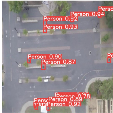
Fig. 3. Example of Yolov5x for person detection.
