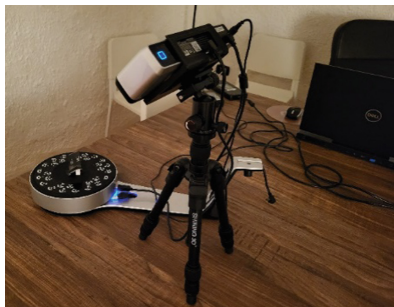
Fig. 4. EinScan SP structured light system 3D scanning system.
