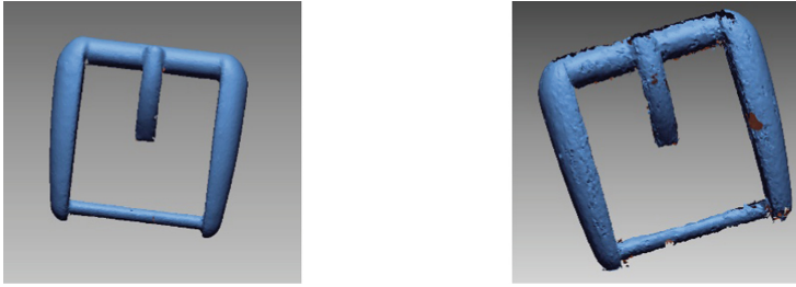
Fig. 2. Surfaces obtained by means of Romer Absolute ARM (left) and NextEngine HD (right) 3d scanners.
