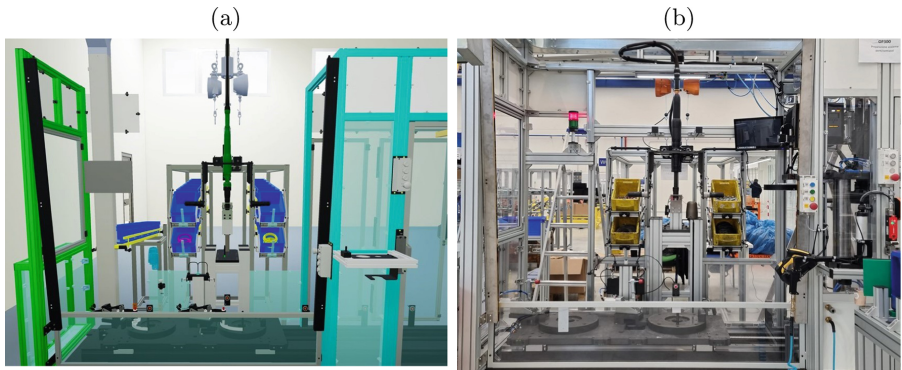
Fig. 3. From VR to reality: versus the corresponding machine virtualized by using the unreal engine platform (a) the rear axle shaft machine assembled in the company plant (b).
