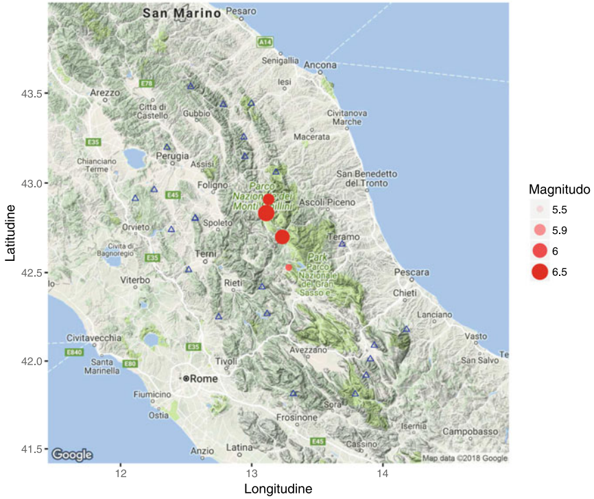
Fig. 2 Geographic coordinates of the seismic events (red points) and seismographs (blue triangle points)
