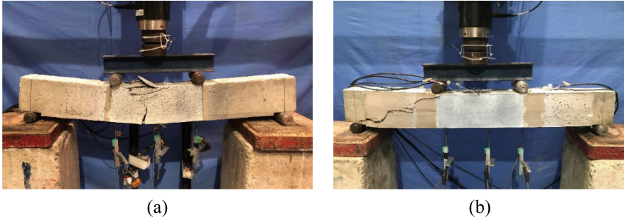
Fig. 2. The externally reinforced beams: flexural failure (a) and the shear failure (b).
