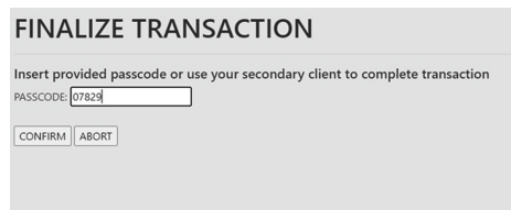
Fig. 9. Screen shown on the PAT to validate the transaction in case of Scenario #2 . If the details of the transaction shown on the AAT match the intended ones, \mathcal{A} can insert the code in the passcode field and press the confirm button to validate the transaction.
