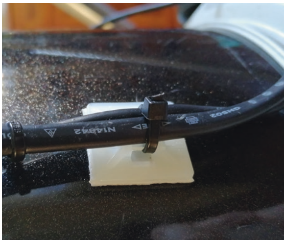
Fig 7.4 A self-adhesive pad and plastic tie wrap used to secure cables to a telescope tube without the need for any cutting or drilling
