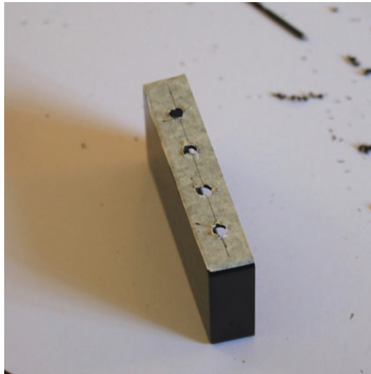
Fig. 12.6 Holes Drilled for all the Plugs and sockets
