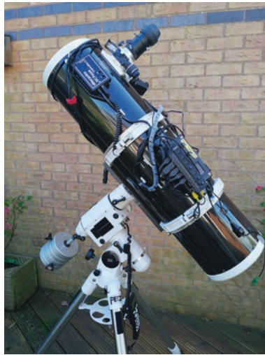
Fig. 4.30 A typical German EQ mount with telescope in the home position
