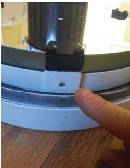
Fig. 10.9 Primary mirror clips and retaining side screws; these must not be over tightened
