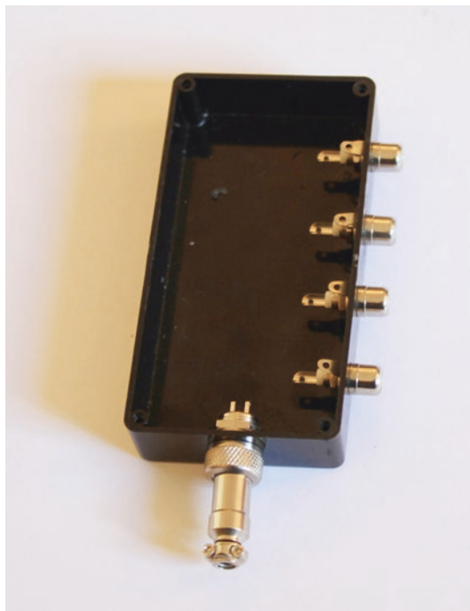
Fig. 12.7 Sockets mounted in project box
