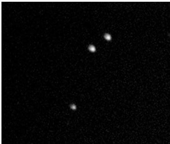
Fig. 10.1 Coma visible in stars at the edge of the FOV
