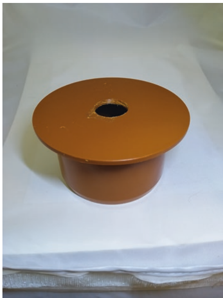
Fig. 12.26 Hole drilled for Camera
