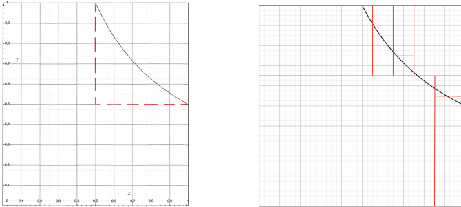
Fig. 1. (left) Class decision lines for (x > 0.5) \wedge (y > 0.5) (dashed) and x * y > 0.5 (solid) and (right) space decomposition by axis-parallel decisions for x * y > 0.5
