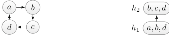
Fig. 1. An AF with the given attack relation (left) and a TD of the framework (right).
