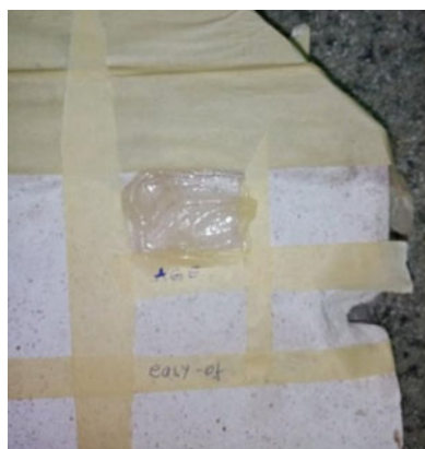
Fig. 17.4 Stone material divided into testing zones before (left) and after the treatment (right); zone 5—steam cleaning + AGE; zone 6—steam cleaning + easy-off solution
