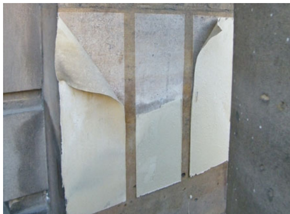
Fig. 19.1 Sample surfaces to determine the optimal application thickness (continuously increasing within an area of 2 mm to 6 mm) or application quantity one day after application. The self-detaching effect at low film thickness is clearly visible. [Photo: Remmers]
