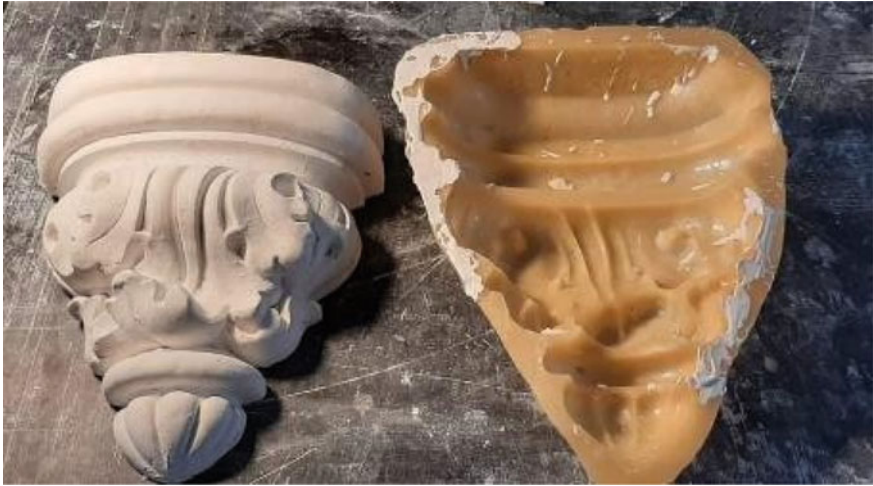
Fig. 14.14 On the left a replica of the corbel and on the right the mold in beeswax
