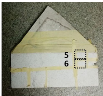
Fig. 17.4 Stone material divided into testing zones before (left) and after the treatment (right); zone 5—steam cleaning + AGE; zone 6—steam cleaning + easy-off solution
