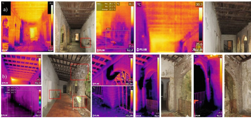
Fig. 7.8 a Thermal imaging of the corridor first level and b second level
