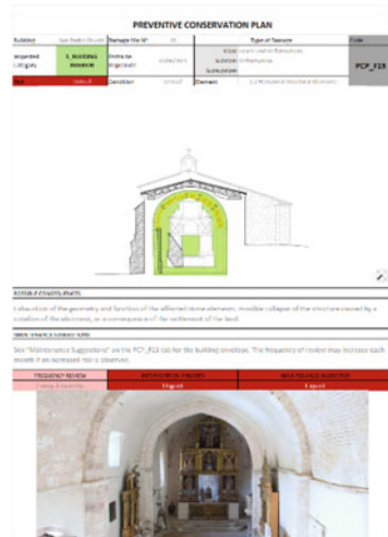
Fig. 6.12 PDF sheets with the damages observed during the inspection: a broken elements (ceramic tiles); and b deformation of the barrel vault
