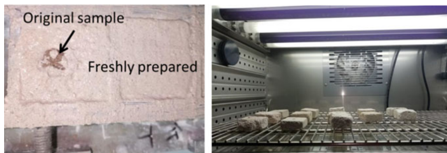
Fig. 18.4 Freshly prepared samples (left) and their artificial ageing in the chamber (right) (Photodocumentation of the MoDeCo2000 project)
