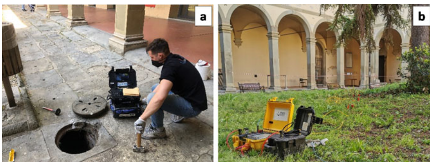
Fig. 13.2 Execution of the investigations inside the Nigetti cloister: a endoscopic investigation inside the pipes found; b geophysical investigations for the characterization of infiltrative phenomena
