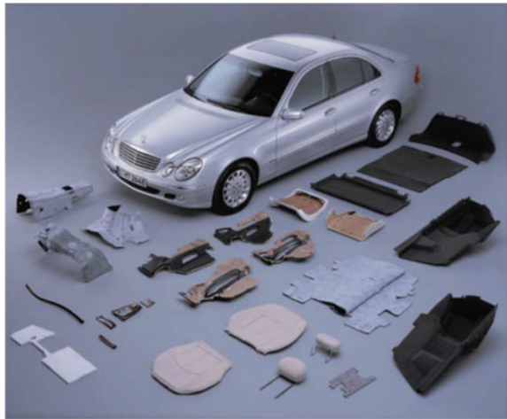
Fig. 1 Application of NFRC on Mercedes Benz E-class components, ranging from floor mats to door panels [2]
