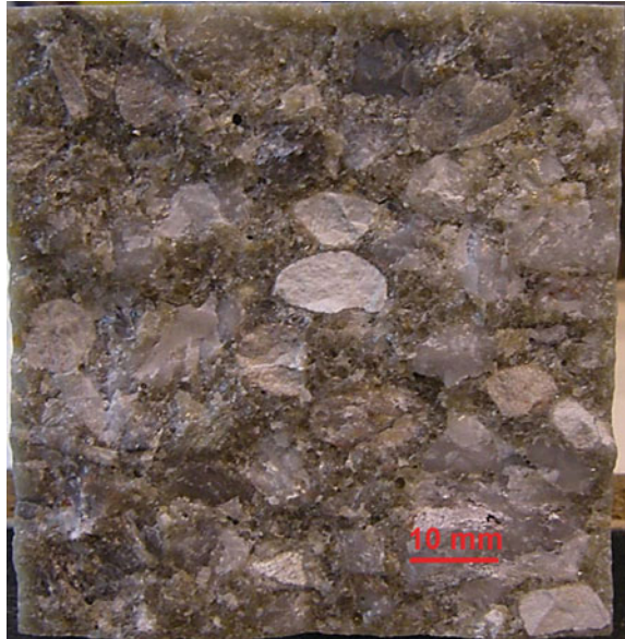
Fig. 2 Broken mineral cast specimen cross section
