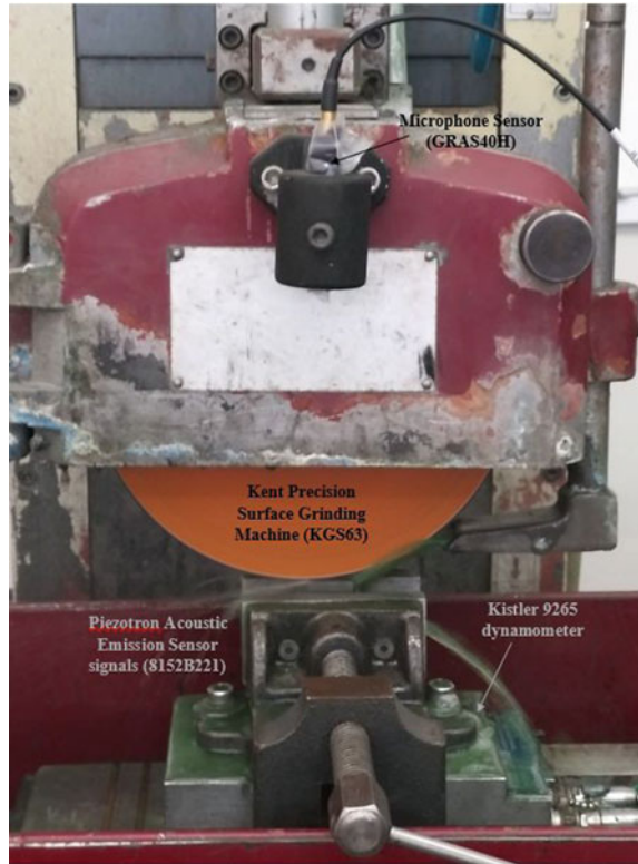
Fig. 1 Experimental setup for grinding test of Ti6Al4v alloy
