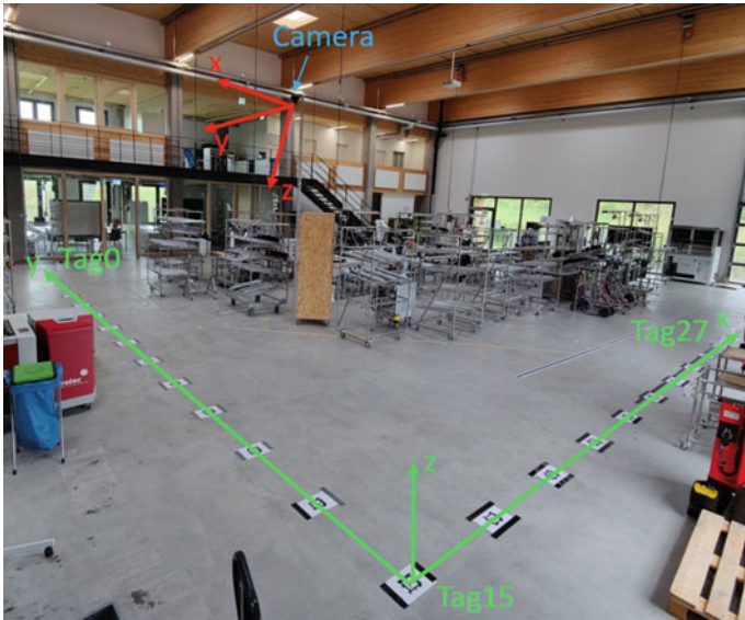
Fig. 2 Test setup using a PTZ camera and AprilTags
