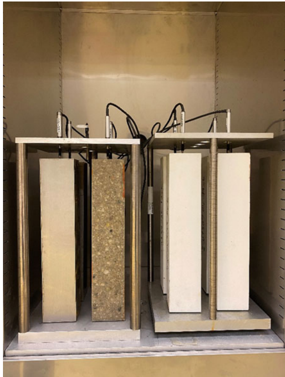
Fig. 7 Drying of the water exposed specimens in the climate chamber
