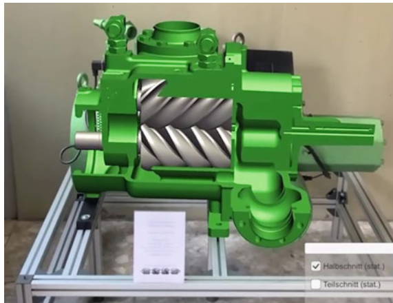
Fig. 4 AR function for the section view
