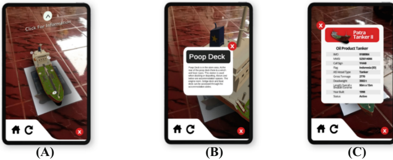
Fig. 2. (A) Main scene after scanning Image target and displaying some world canvas-based button to display information. (B) The main scene when displaying detail Information based on screen canvas. (C) The main scene when displaying specification information based on screen canvas.
