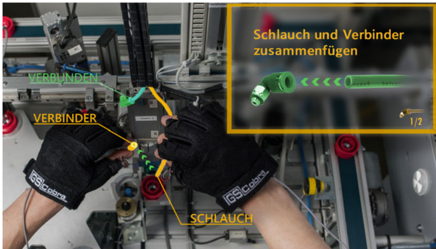
Fig. 1 Example of using the AR assistant for assembly of the plants’ components
