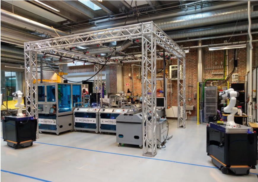
Fig. 3 Picture of two of the MIR AMRs integrated and operated with 5G technology at the AAU 5G Smart Production Lab, Aalborg University, Denmark
