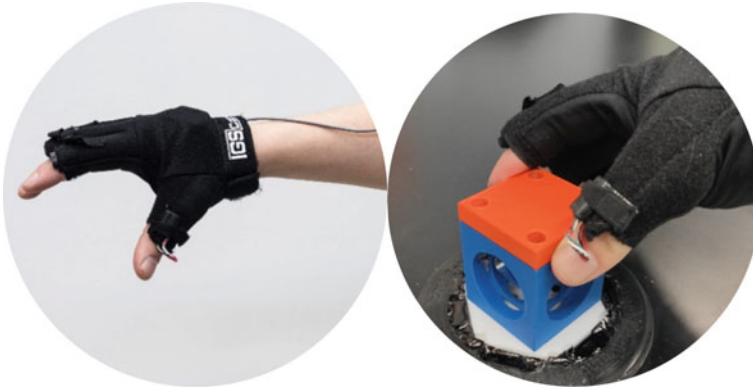
Fig. 4 Data glove as an assistance system input device for assembly recognition (left) and grasping of assembly part “cover” (right)
