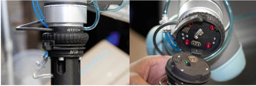
Fig. 3 “Tool changer” from 4tech. Left = AM part fitted on a Universal Robot; Right = disassembled AM part showing complex and flexible internal structure
