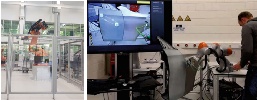
Fig. 2 Comparison of a robot versus a cobot. From the left to the right: (1) isolated robot working surrounded by fences and (2) collaborative robot working along side a human worker without physical separation
