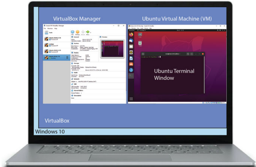
Fig. 11.7: The Ubuntu Virtual Machine (VM) running on a Windows 10 Laptop (illustration). The VirtualBox Manager is what opens when you run VirtualBox. The Ubuntu Virtual Machine (VM) is installed and opened from within the VirtualBox Manager. The Ubuntu Terminal Window is opened from within the Ubuntu VM and is where Ubuntu VM Linux commands are entered
