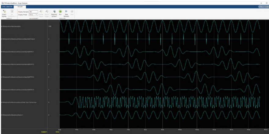
Fig. 3.16: Using the Simulink Logic Analyzer to debug the system with cosine wave. During initial development, overflow occurred in the add unit of the overlap and add section resulting in a non-sinusoidal output (the second line from bottom). The correct output is the bottom waveform
