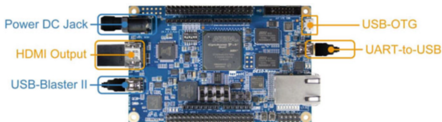
Fig. 11.1: The USB UART connection is on the right side, above the Ethernet port. It uses a USB Mini-B Connector. Figure is from the DE10-Nano getting started guide
