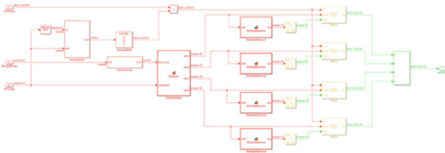
Fig. 3.15: The contents of the overlapAdd block that assembles the time domain FFT frames. Note: Open the model fftAnalysisSynthesis.slx in Simulink for better viewing ( GitHub link )
