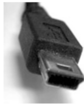
Fig. 11.3: The USB Mini-B connector
